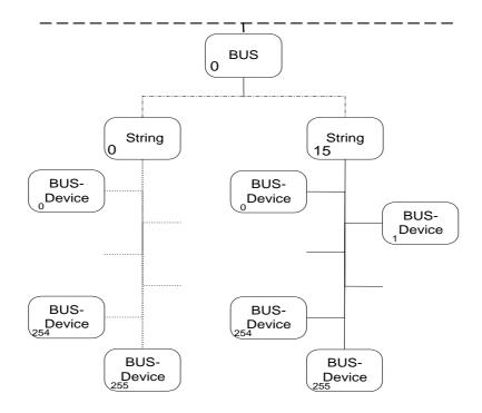
Each participant of the network possesses a unique network address, which consists of a bus address, a string address and a device address. With this type of addressing, 256 devices can be addressed per logic string. At a maximum of 16 strings this results in an address range of up to 4096 (16 x 256) devices. The bus address serves for the separation of neighbouring plants (maximum 15).
