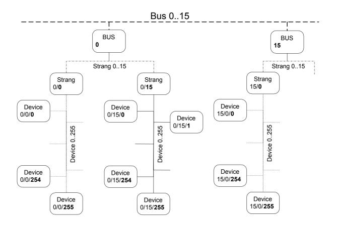
Each network participant has a unique network address composed of a bus address, a network address, a string address and a device address. 256 devices per logical string can be addressed by this address mode resulting in an address range of up to 4096 devices in case of a maximum of 16 strings. Contiguous plants (a maximum of 15) are separated by the bus address.
