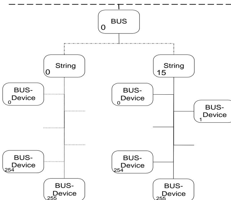
Each participant of the network possesses a unique network address, which consists of a bus address, a string address and a device address. With this type of addressing, 256 devices can be addressed per logic string. At a maximum of 16 strings this results in an address range of up to 4096 ( $16 \times 256$ ) devices. The bus address serves for the separation of neighbouring plants (maximum 15).
