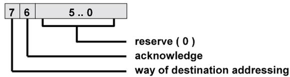
Bit 7: This bit selects the kind of the destination address. If it is set, the destination address is a group address, otherwise the destination address is a network address.
